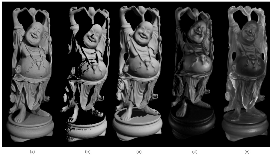
Figure 23.17. 3D Fax of a statuette of a Buddha. From left to right: photograph of the statuette; range image; integrated 3D model; model after hole filling; physical model obtained via stereolithography. Reprinted from [?], Figure 10.
