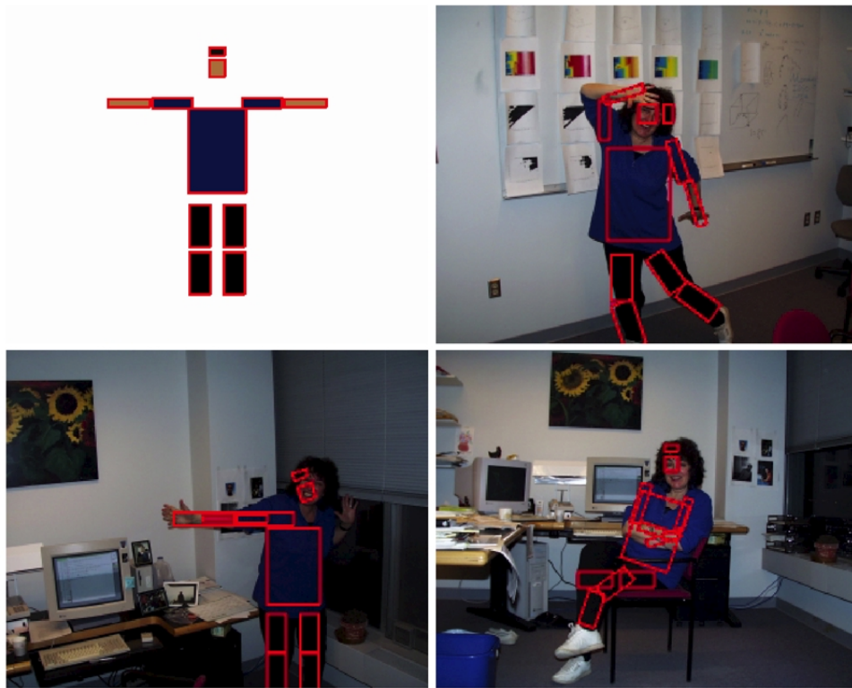
Figure 21.21. On the top left , a tree structured model of a person. Each segment is coloured with the image colour expected within this segment. The model attempts to find a configuration of these 11 body segments (9 limb segments, face and hair) that (a) matches these colours and (b) is configured like a person. This can be done with dynamic programming, as described in the text. The other three frames show matches obtained using the method. figure from Efficient Matching of Pictorial Structures P. Felzenszwalb and D.P. Huttenlocher p.8, in the fervent hope of receiving permission
