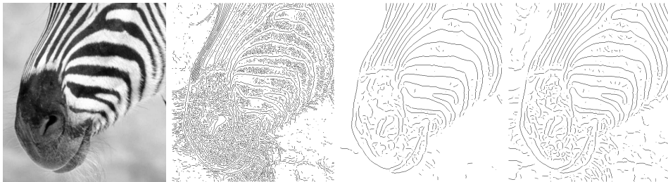
Figure 8.15. Edge points marked on the pixel grid for the image shown on the left . The edge points on the center left are obtained using a Gaussian smoothing filter at \sigma one pixel and gradient magnitude has been tested against a high threshold to determine whether a point is an edge point or not. The edge points on the center right are obtained using a Gaussian smoothing filter at \sigma four pixels and gradient magnitude has been tested against a high threshold to determine whether a point is an edge point or not. The edge points on the right are obtained using a Gaussian smoothing filter at \sigma four pixels and gradient magnitude has been tested against a low threshold to determine whether a point is an edge point or not. At a fine scale, fine detail at high contrast generates edge points, which disappear at the coarser scale. When the threshold is high, curves of edge points are often broken because the gradient magnitude dips below the threshold; for the low threshold, a variety of new edge points of dubious significance are introduced.
