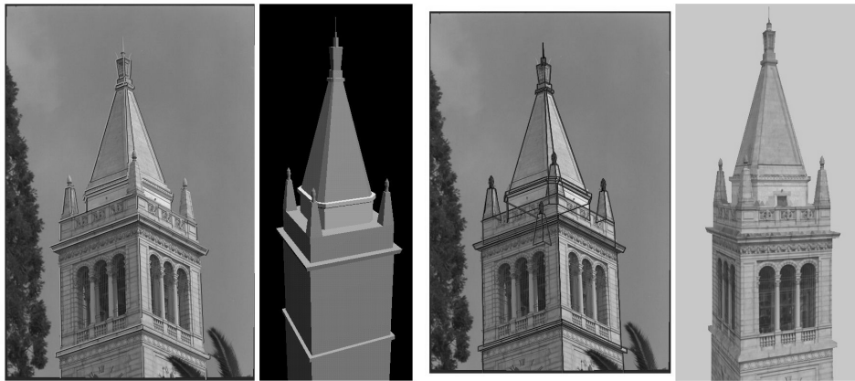
Figure 25.10. Façade model of the Berkeley Campanile. From left to right: a photograph of the Campanile, with selected edges overlaid; the 3D model recovered by photogrammetric modeling; reprojection of the models into the photograph; a texture-mapped view of the model. Reprinted from [?], Figure 2.
