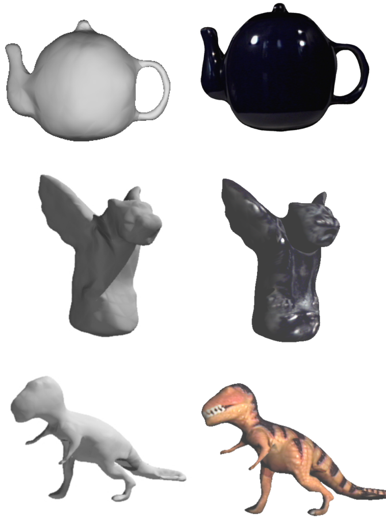
Figure 25.6. Shaded and texture-mapped models of a teapot, a gargoyle and a dinosaur. The teapot was constructed from six registered photographs; the gargoyle and the dinosaur models were each built from nine images. Reprinted from [?], Figures 4 and 5.
