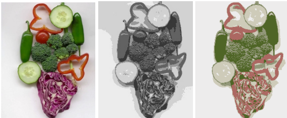
Figure 15.15. On the left, an image of mixed vegetables, which is segmented using k -means to produce the images at center and on the right. We have replaced each pixel with the mean value of its cluster; the result is somewhat like an adaptive requantization, as one would expect. In the center, a segmentation obtained using only the intensity information. At the right, a segmentation obtained using colour information. Each segmentation assumes five clusters.
