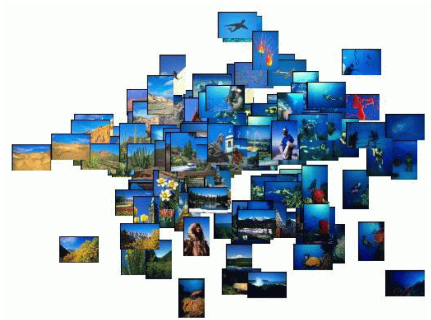
Figure 24.7. Images laid out according to their similarity using the earth mover's distance (EMD). The EMD can be computed very fast so that displays like this — where distances between images on the display reflect the EMDs between them as faithfully as possible — can be created online. Large numbers of pictures returned from a query into an image database can thus be viewed at a glance, and a mouse click in the neighborhood of pictures that look similar to what the user is looking for tells the retrieval system where to search next. With this technology, users browse and navigate in an image database, just as they would browse through a department store. Because of the large number of images displayed, and their spatially intuitive layout, users quickly form a mental model of what is in the database, and rapidly learn where to find the pictures they need. More information on the EMD can be found in [?]; figure by kind permission of C. Tomasi. Permission granted for Library Trends article; reproduced in the fervent hope that permission will be granted for the book, too
