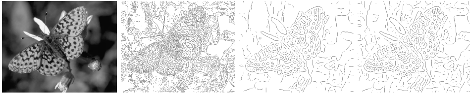
Figure 8.14. Edge points marked on the pixel grid for the image shown on the left . The edge points on the center left are obtained using a Gaussian smoothing filter at \sigma one pixel and gradient magnitude has been tested against a high threshold to determine whether a point is an edge point or not. The edge points on the center right are obtained using a Gaussian smoothing filter at \sigma four pixels and gradient magnitude has been tested against a high threshold to determine whether a point is an edge point or not. The edge points on the right are obtained using a Gaussian smoothing filter at \sigma four pixels and gradient magnitude has been tested against a low threshold to determine whether a point is an edge point or not. At a fine scale, fine detail at high contrast generates edge points, which disappear at the coarser scale. When the threshold is high, curves of edge points are often broken because the gradient magnitude dips below the threshold; for the low threshold, a variety of new edge points of dubious significance are introduced.
