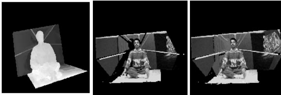
Figure 25.8. Multi-baseline stereo. From left to right: the range map associated with a cluster of cameras; a texture-mapped image of the corresponding mesh, observed from a different viewpoint; note the dark areas associated with depth discontinuities in the map; a texture-mapped image constructed from two adjacent camera clusters; note that the gaps have been filled. Reprinted from [?], Figures 3 and 8.
